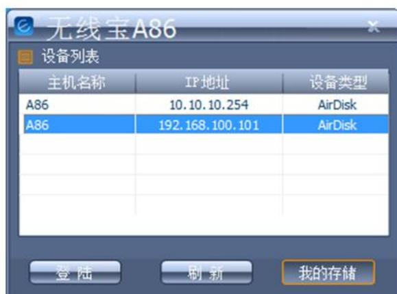
Without installation need for Mac OS/PC clients, A86 can be used by double-clicking or accessed by directly entering 10.10.10.254 in the browser and entering into the WEB management interface.
